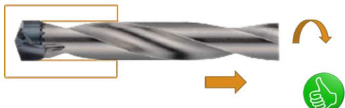
When the required depth is reached, retract the drill by 0.1 to 0.5mm and reduce to 500 rpm followed by a complete retraction with normal feed.
