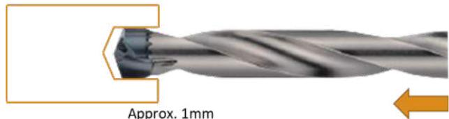
Enter the pilot hole with the 12xD body running a maximum of 500 rpm, up to 1mm above the depth drilled with the pre-drill.
